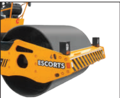
Compaction Force Highest total compaction force, static linear load and amplitude reduces the number of passes required to achieve the desired compaction.
