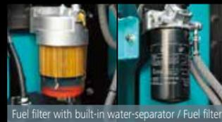
Fuel filter with built-in water-separator / Fuel filter
