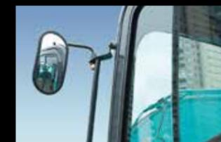
Greater safety assured by rearview mirrors on left and right, and a third mirror mounted at lower right.
