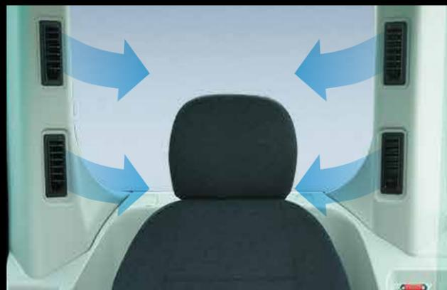
The large air-conditioner has vents on the back pillars that blow from behind and to the right and left of the operator's seat. They can be adjusted to put a direct flow of cool/warm air on the operator, which means a more comfortable operating environment.
