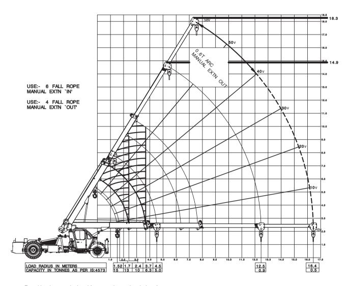
Rated loads are calculated for operation on leveled surface.
