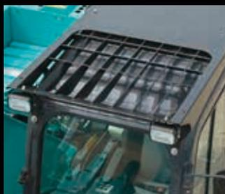
The top guard (FOPS, Top Guard Level II. (Meets ISO10262)) provided as option. The top-mounted working light ensures a wide field of view.
