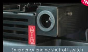
Emergency engine shut-off switch
