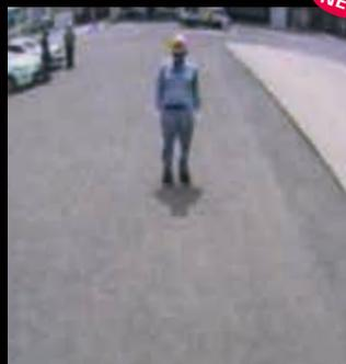
A rear view camera is installed as option to simplify checking for safety behind the machine. The picture appears on the color monitor.
