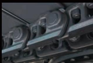
The durability of the track link is increased compared to SK500HDL-8.
