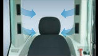
The large air-conditioner has louvers on the back pillars that blow from behind and to the right and left of the operator's seat. They can be adjusted to put a direct flow of cool/warm air on the operator, which means a more comfortable operating environment.
