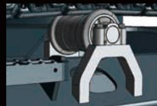
Double-support outer flanged upper rollers can withstand powerful vibrations.
