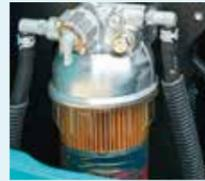
Pre fuel filter with built-in water separator
