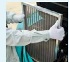
removed and cleaned without the use of tools.
