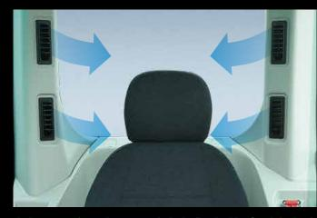
The large air-conditioner has vents on the back pillars that blow from behind and to the right and left of the operator's seat. They can be adjusted to put a direct flow of cool/warm air on the operator, which means a more comfortable operating environment.
