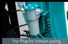
The filter for breaker piping
