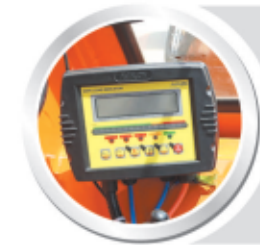
SLI Monitoring System
